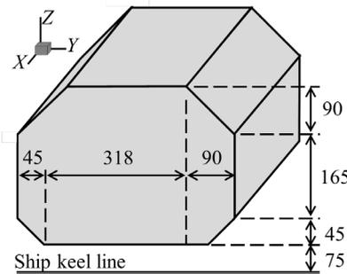
(b) Dimension of inner tank (unit: mm)
