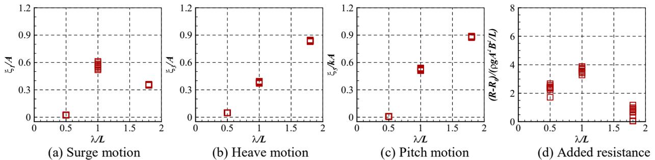
Fig. 2 Repeat results on ship motion RAOs and added resistance (10 repeats,  $0.5H_0$  filling tank, wave height  $H/L=0.008$ , ship  $Fn=0.2$ )
