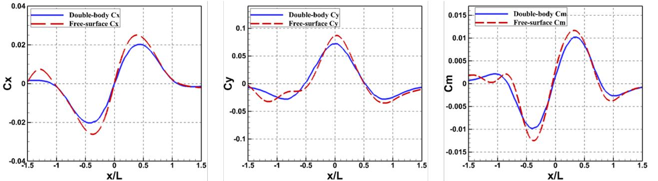
Fig. 2 X-direction, y-direction forces and moment according to the horizontal distance
