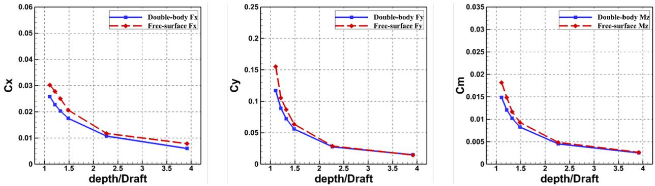
Fig. 6 Force coefficients for the different depth-draft ratio
