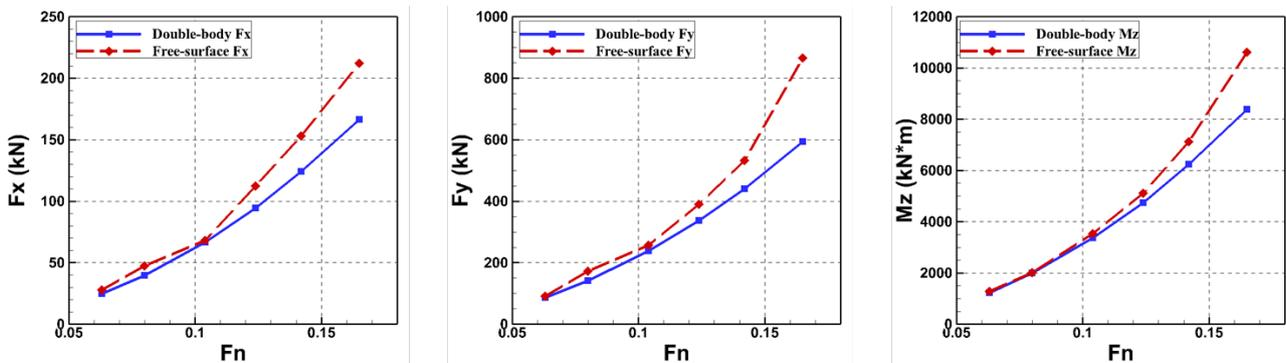
Fig. 4 Passing ship loads according to passing ship speed
