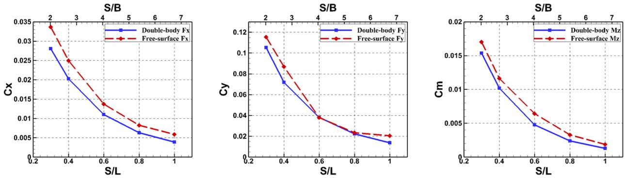
Fig. 5 Force coefficients for difference separation distances
