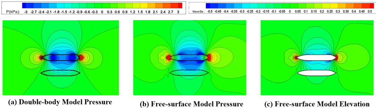
Fig. 3 Pressure fields of Double-body and Free-surface model at  $x/L$  of zero ( $F_n$ : 0.142)
