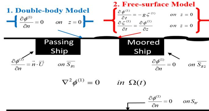
Fig. 1 Linear boundary value problem for Double-body model and Free-surface model
